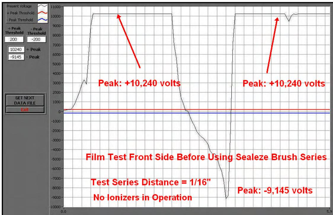
The first test series was conducted by positioning one of the Sealeze™ brushes over the Front Side of the PETG film and below the Back Side of the substrate at a distance of approximately 1/16<sup>th</sup> of an inch. **Figure 13** is an illustration of the brush positioning.
