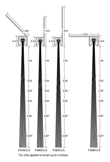
**SEALEZE**° nylon Therm-L-Brush up to 4 inches long are UL labeled for use on 3-hour fire doors.
